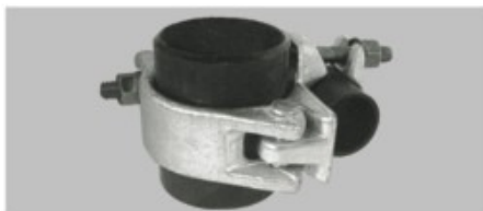
ES-009 COMBINATION DOUBLE COUPLER For Tube OD : 76.1 & 48.3mm Weight : 2.40 kg.
