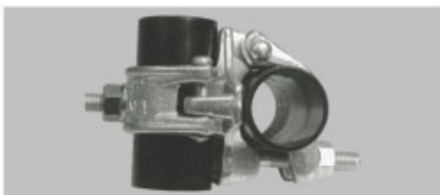
ES-003 DOUBLE COUPLER (HEAVY DUTY) For Tube OD : 48.3mm Weight : 1.25 kg.
