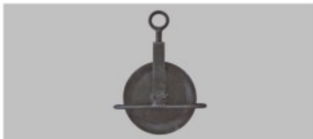
ESP-07 GIN WHEEL Sheave Dia : 30cm Rope Dia : 20mm Weight : 5.80 kg. Capacity : 250 kg.
