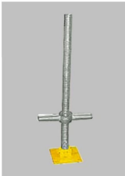
EJS-02 SWIVEL ADJUSTABLE BASE JACK PIPE OD 38mm, 35mm, 34mm, SIZE : 450mm, 500mm, 610mm, 700mm
