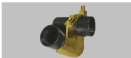
ES-029 PUTLOG COUPLER For Tube OD : 48.3mm Weight : 0.73 kg.
