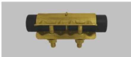
ES-032 SLEEVE COUPLER For Tube OD : 48.3mm Weight : 1.00 kg.
