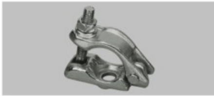
ES-015 SINGLE COUPLER For Tube OD : 48.3mm Weight : 0.87 kg.
