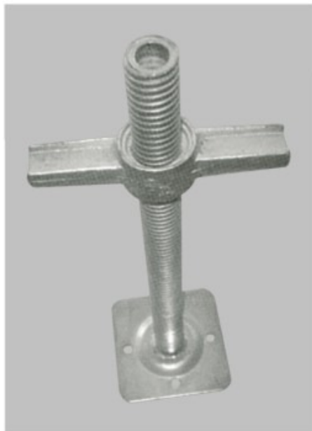
EJS-01 ADJUSTABLE BASE JACK PIPE OD 38mm, 35mm, 34mm, SIZE : 450mm, 500mm, 610mm, 700mm
